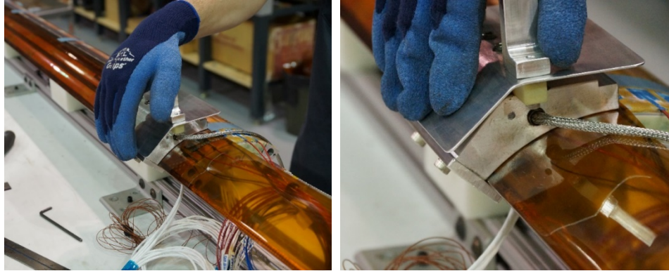
Figure 22: Hot iron to bond the Kapton to the coil
