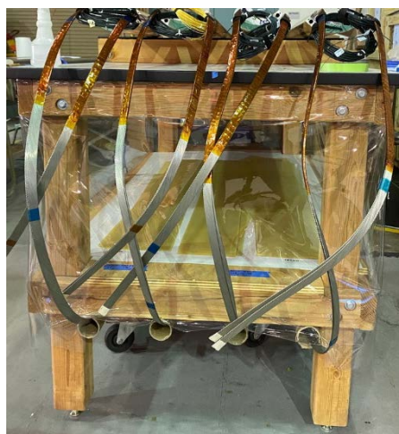
Figure 1: Coils on table with leads tucked into tubes under the table
