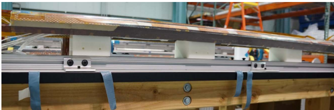
Figure 13: Coil mounted for ground plane installation
