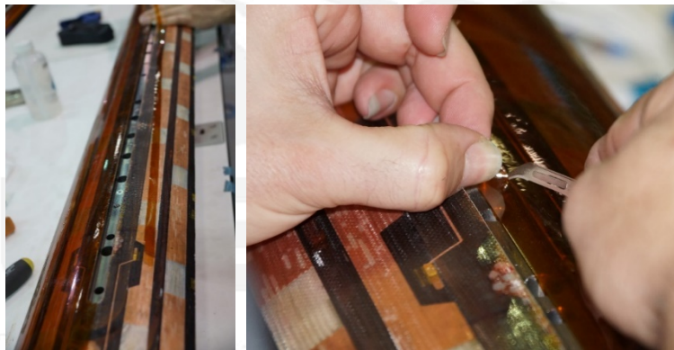
Figure 23: Trim the Kapton away from the center groove
