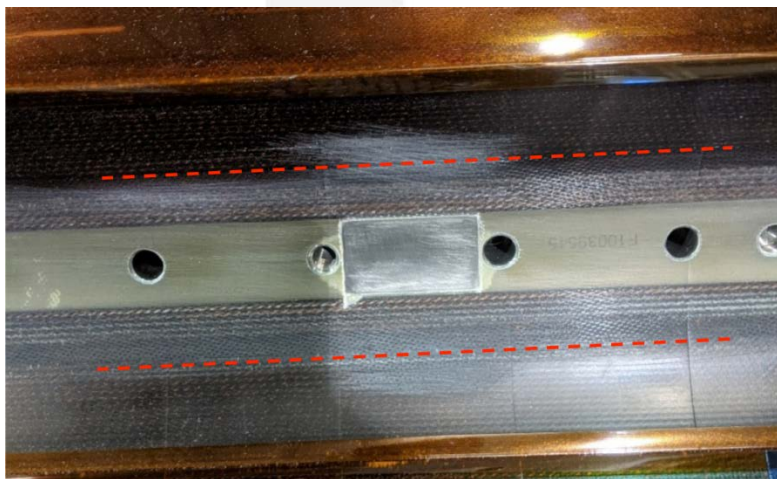
Figure 5: cut out a section of epoxy
