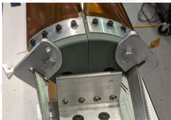
Figure 14: Fixtures to capture coil leads
