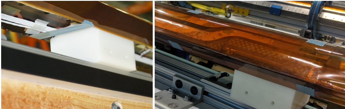
Figure 19: Tape the Kapton in place. Use 3M 8979 tape.
