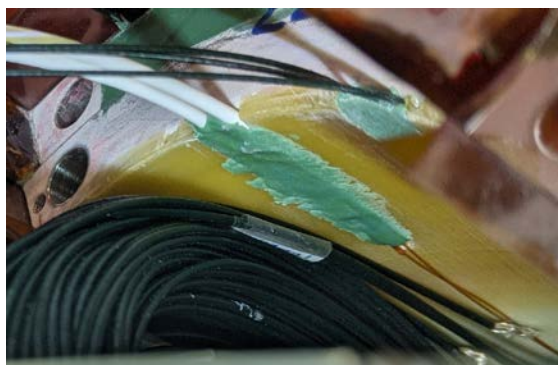
Figure 12: Green putty securing the fiber
