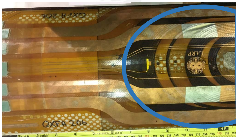
Figure 21: Do not iron the cable turns
