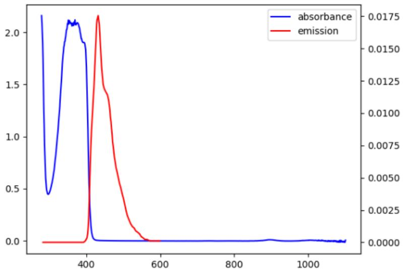
We determined  $\epsilon c = A_0 / I_0$  using the experimental data  $A_0$  (assuming  $I_0 = 4\text{mm}$ ) an reconstructed for any distance using Beer-Lambert Law  $T = 10^{-A} = 10^{-\epsilon cl}$ .
