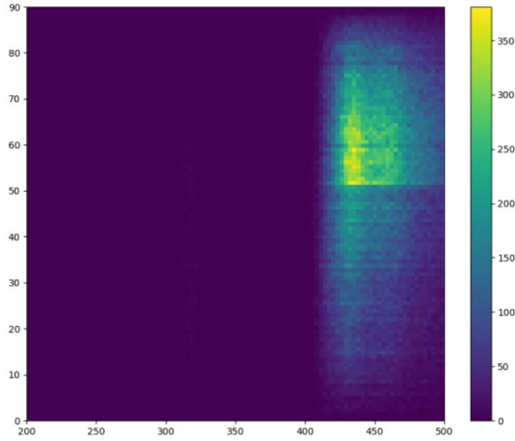
Megacell. Histogram of photons escaped through dichroic filters coming from inside the X-ARAPUCA (wl x inc. angle). Border = 0.1, Dimple Radius = 0.5
