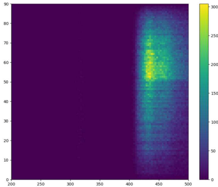
Supercell. Histogram of photons escaped through dichroic filters coming from inside the X-ARAPUCA (wl x inc. angle). Border = 0.1, Dimple Radius = 1.5
