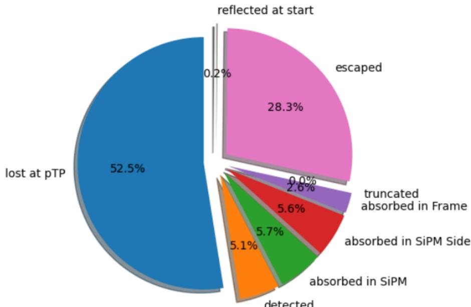
X-ARAPUCAS Supercells with dimples and SiPMs with thin sides. Dimples with radius 4.3mm, without thin sides.
