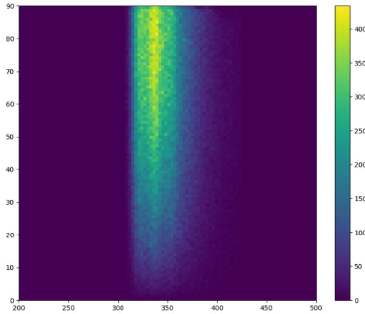
Supercell. Histogram of photons escaped through dichroic filters coming from inside the X-ARAPUCA (wl x inc. angle). Border = 0.1, Dimple Radius = 0
