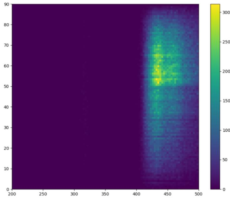
Supercell. Histogram of photons escaped through dichroic filters coming from inside the X-ARAPUCA (wl x inc. angle). Border = 0.1, Dimple Radius = 2
