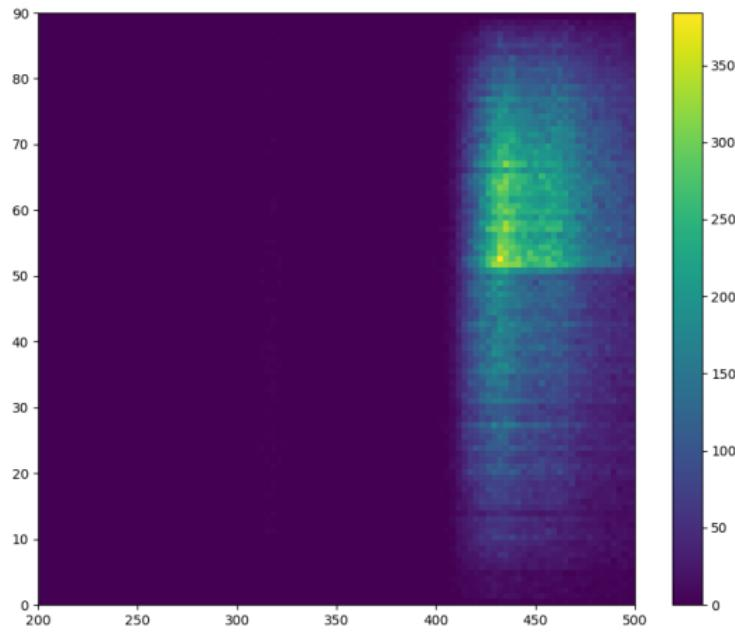
Megacell. Histogram of photons escaped through dichroic filters coming from inside the X-ARAPUCA (wl x inc. angle). Border = 0.1, Dimple Radius = 1.5
