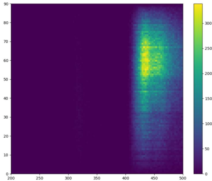
Supercell. Histogram of photons escaped through dichroic filters coming from inside the X-ARAPUCA (wl x inc. angle). Border = 0.1, Dimple Radius = 0.5
