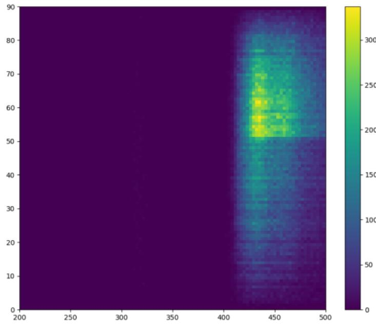
Megacell. Histogram of photons escaped through dichroic filters coming from inside the X-ARAPUCA (wl x inc. angle). Border = 0.1, Dimple Radius = 2
