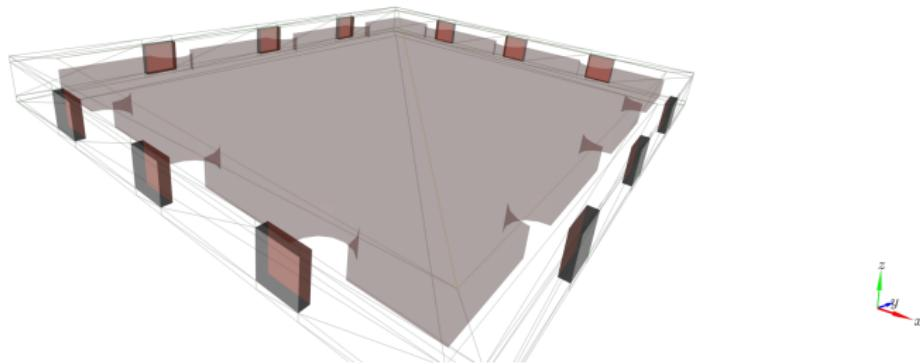
X-ARAPUCAS Supercells with dimples and SiPMs with thin sides. Dimples with radius 4.3mm and thin sides of 1.4mm.
