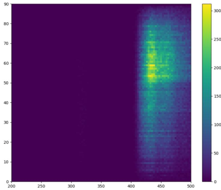
Supercell. Histogram of photons escaped through dichroic filters coming from inside the X-ARAPUCA (wl x inc. angle). Border = 0.1, Dimple Radius = 1
