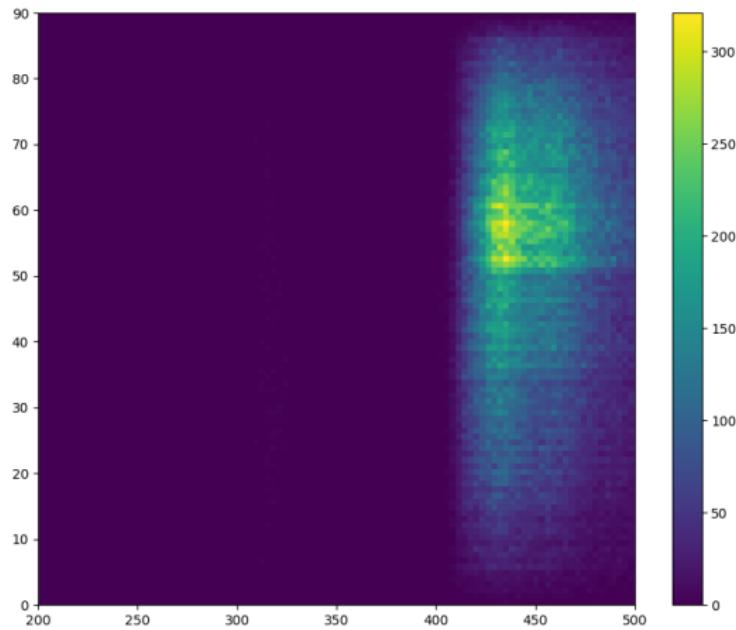
Supercell. Histogram of photons escaped through dichroic filters coming from inside the X-ARAPUCA (wl x inc. angle). Border = 0.1, Dimple Radius = 3
