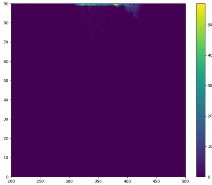
Supercell. Histogram of photons that actually enter the X-ARAPUCA (wavelength x incidence angle). Border = 0.1, Dimple Radius = 1.5
