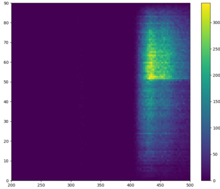
Megacell. Histogram of photons escaped through dichroic filters coming from inside the X-ARAPUCA (wl x inc. angle). Border = 0.1, Dimple Radius = 1
