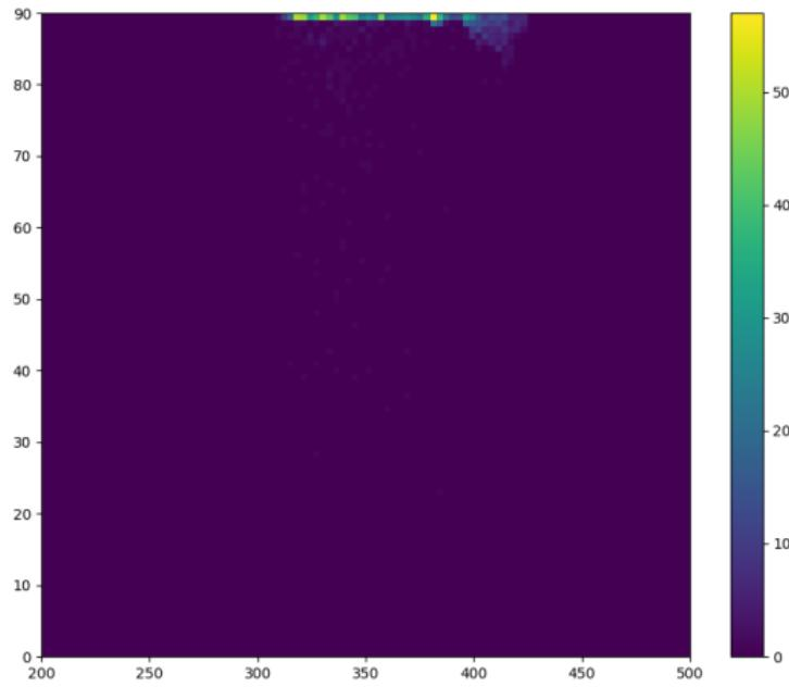
Megacell. Histogram of photons that actually enter the X-ARAPUCA (wavelength x incidence angle). Border = 0.1, Dimple Radius = 0.5
