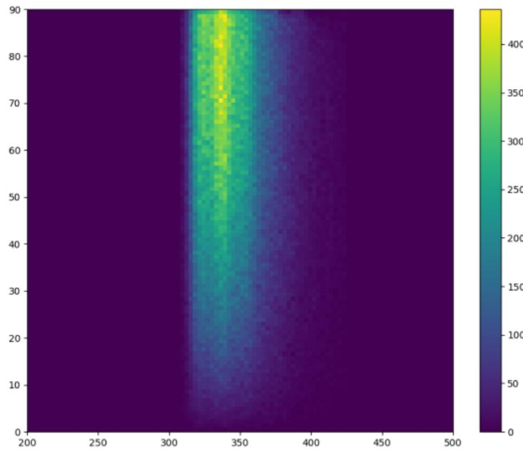
Megacell. Histogram of photons escaped through dichroic filters coming from inside the X-ARAPUCA (wl x inc. angle). Border = 0.1, Dimple Radius = 0
