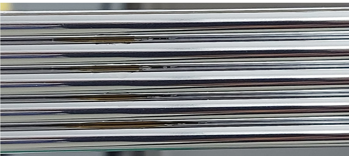
Straws glued together with epoxy ELK5 (~ 20cm spacing)
