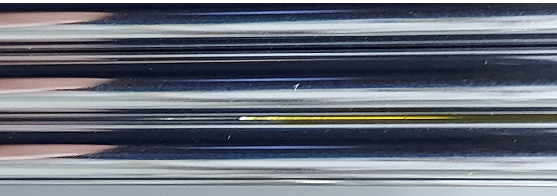
Straws glued together with epoxy ELK5 (~ 20cm spacing)
