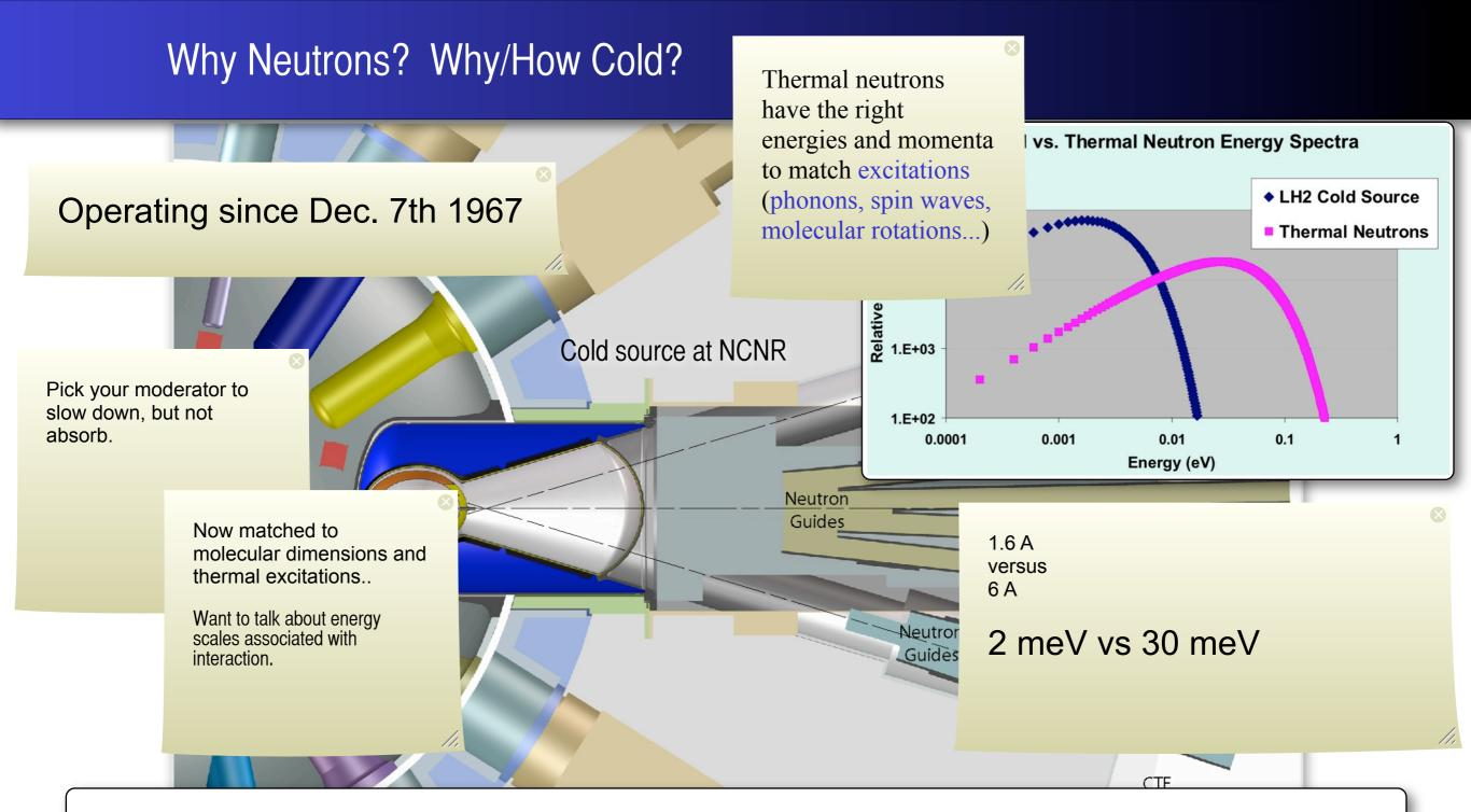
Neutrons partially thermalize in a cold source
