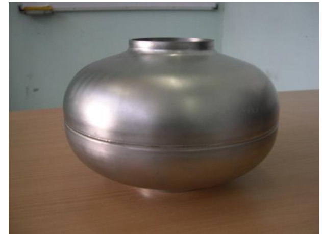
Laser welded half cells of SC Cavity at CMEL,RRCAT
