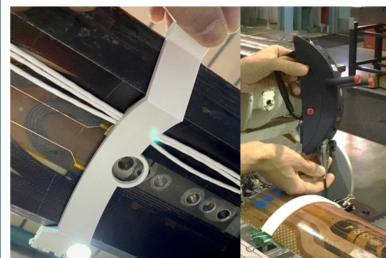
(Left) Fixture for guiding the T-probe with a circle around the pole inner diameter to acquire more points (Right) T-probe guided by fixture
