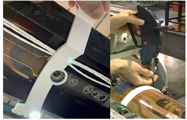
Fig. 3. (Left) Fixture for guiding the T-probe with a circle around the pole inner diameter to acquire more points (Right) T-probe guided by fixture
