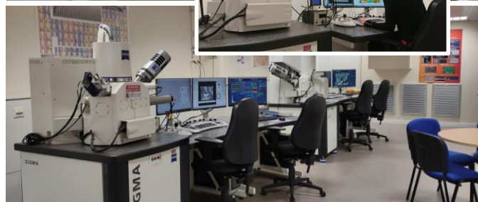
Advanced electron microscopy including FIB-SEM and a wide range of detectors (EDS, EBSD, low voltage EDS)
