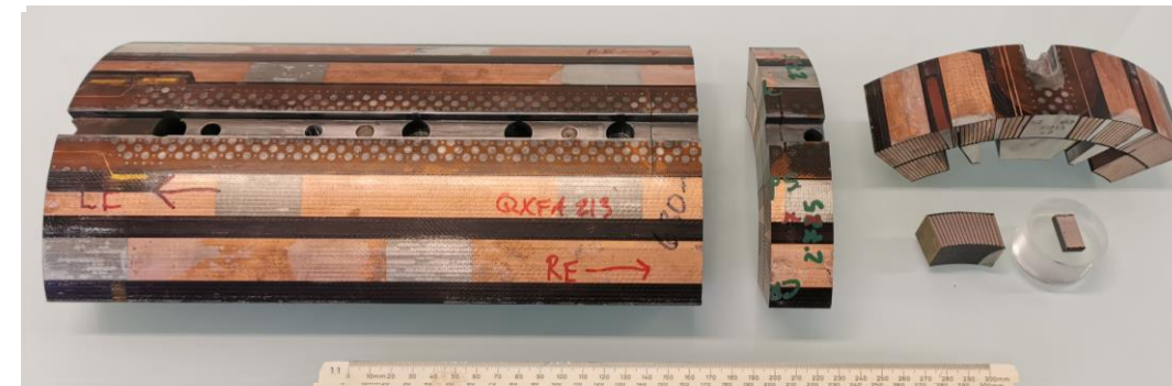
Samples issued from the 4.2 m long AUP 213 coil of the MQXFA08 magnet ↓
