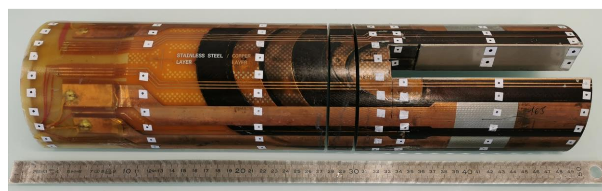
↑ Short model 11 T dipole coil C122 (coil head), connection side
