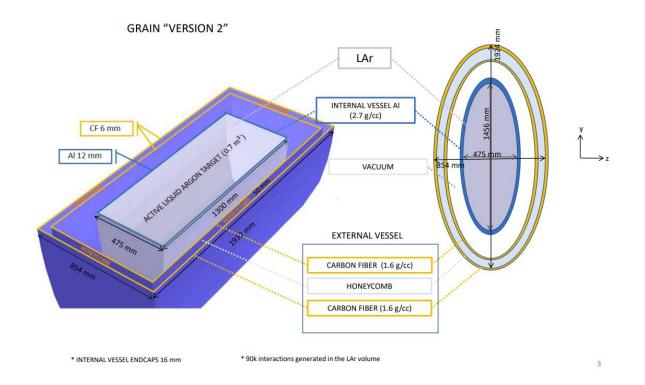
ANALYSIS: The stopping power of each layer is evaluated on 4 classes of primary particles:  $\mu$ , protons, neutron,  $\pi^{+/-}$ . Each of these particles are then classified, from the MC truth, depending on the vessel/volume they stop. A track originated in the LAr volume indeed could stop in one of the following volumes:
