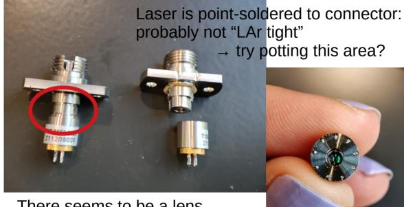
There seems to be a lens inside → usually the laser beam has a focus point ~few mm from lens
