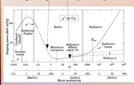
dE/dx for positive muons in Copper K. Nakamura et al. (Particle Data Group), J. Phys. G 37, 075021 (2010)
