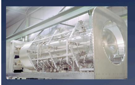
Magnetic horn with reversible polarity focuses either neutrino or anti-neutrino parent mesons
