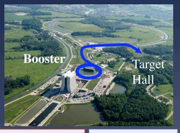
8.9 GeV/c momentum protons extracted from Booster, steered toward a Beryllium target in bunches of 5 × 10<sup>12</sup> at a maximum rate of 5 Hz
