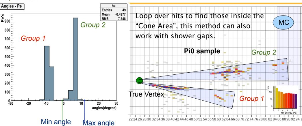
Every group (particle) inside the histogram will have a minimum angle and maximum angle
