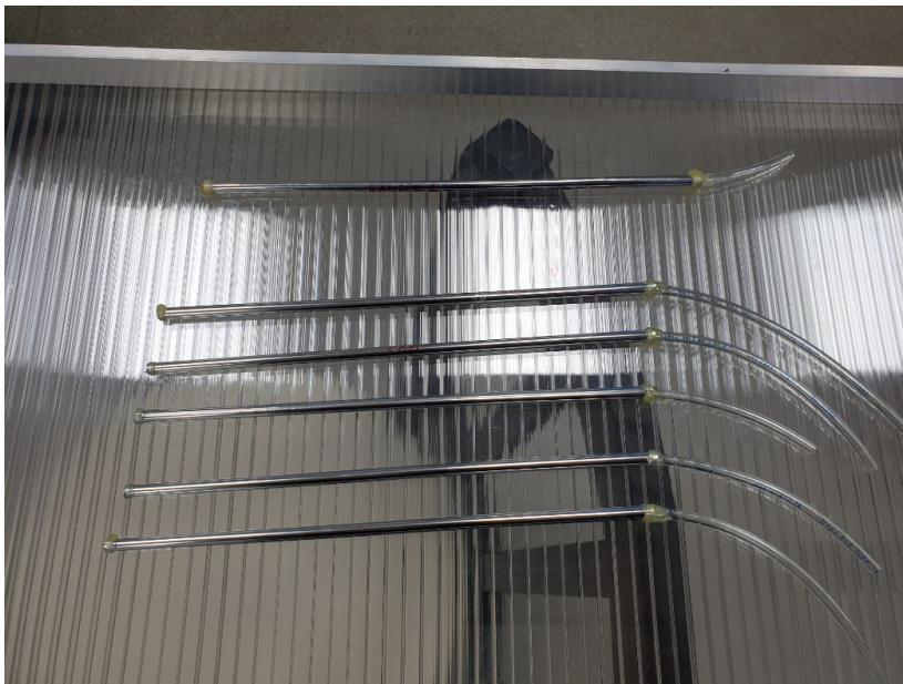
1.1 m long straws produced by GTU for moekup assembly
