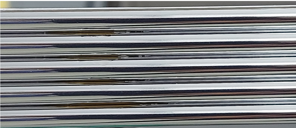
Straws glued together with epoxy ELK5 (~ 20cm spacing)
