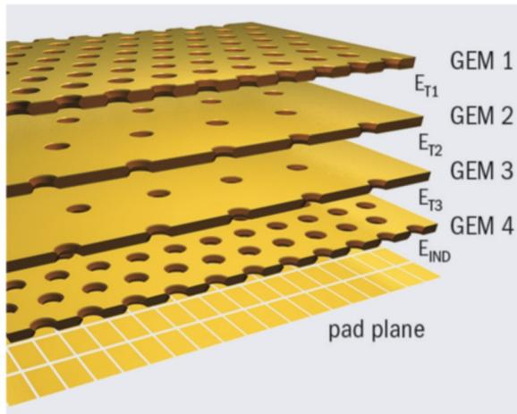
Fig. 1: Schematic view of a stack of four large-size GEM foils as employed for the upgrade of the ALICE TPC
