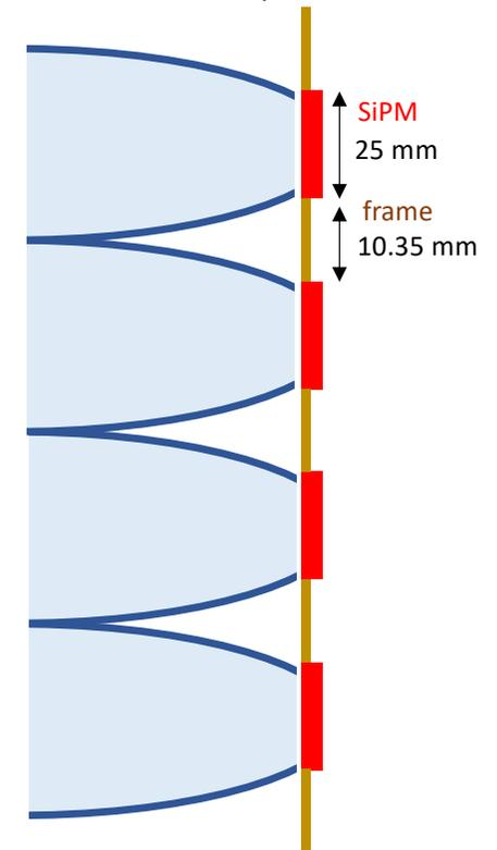
Scheme of a cone (side view, not to scale)
