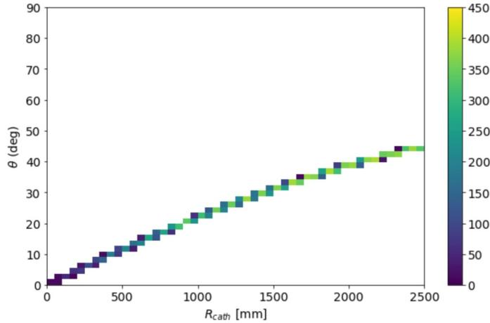
Only direct light reaches the photosensor plane, there is no reflected light
