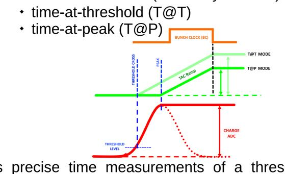
Though VMM3/3a implements precise time measurements of a threshold crossing (T@T), the most of applications measure signal peak time (T@P)
