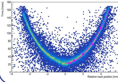
The distance between the track and anode wire is obtained from a measured or simulated *r*(*time*<sub>drift</sub>) dependence.
