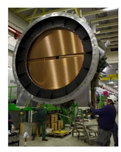
A number of operating and future experiments use Straw Tube detectors for precise tracking. Small material budget and achievable large acceptance make Straw Tube Trackers attractive for such future facilities like Near Detector complex of the DUNE [1] experiment, the Spectrometer Straw Tracker of the SHiP [2] experiment, and Straw Tracker of the SPD [3] experiment.
