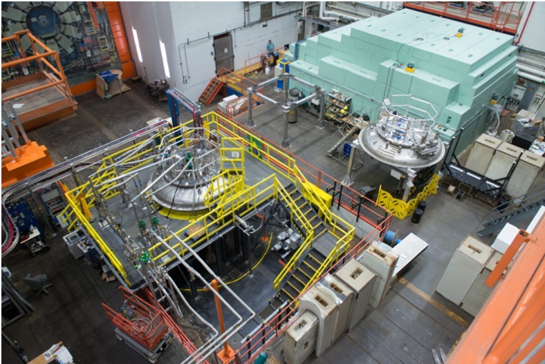
Fermilab SQMS is constructing a world record sized DR capable of hosting thousands of qubits
