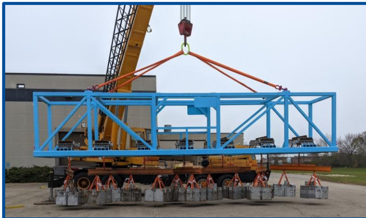
32-tonne load test @ FNAL – Jan 22
