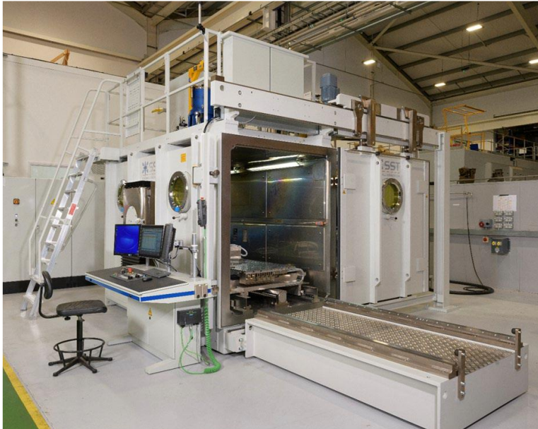
New Steigerwald Electron Beam Welder installed and commissioned at TWI (Dec 2020)
