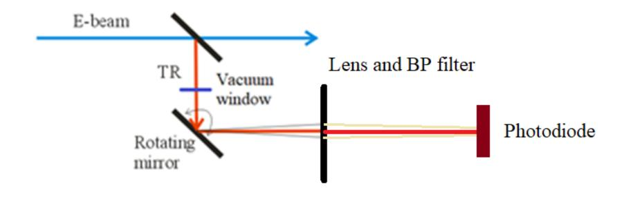
• Proposed optical band: 0.5 - ~2 um (measure in ~100 nm steps)
