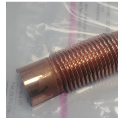
Bubbles under Cu coating (no bubbles where penetrant compound applied)
