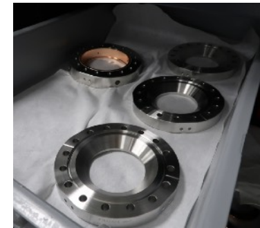
All pics : air side outer cond. test piece and parts
