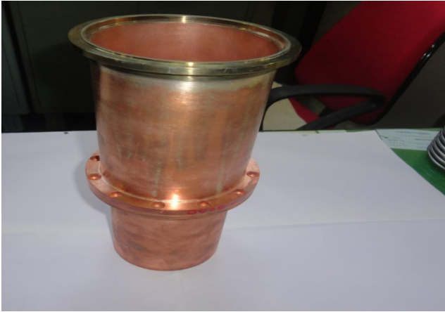
650 MHz Outer conductor Extension ( Bellow EM shield design)
