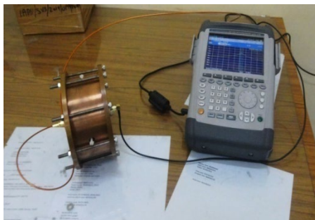
Alumina loss tangent measurement set-up developed at BARC
