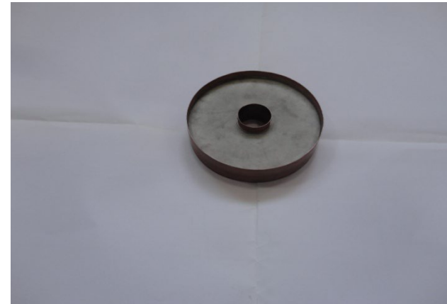
Alumina disc after brazing to copper sleeves ( discoloration observed)
