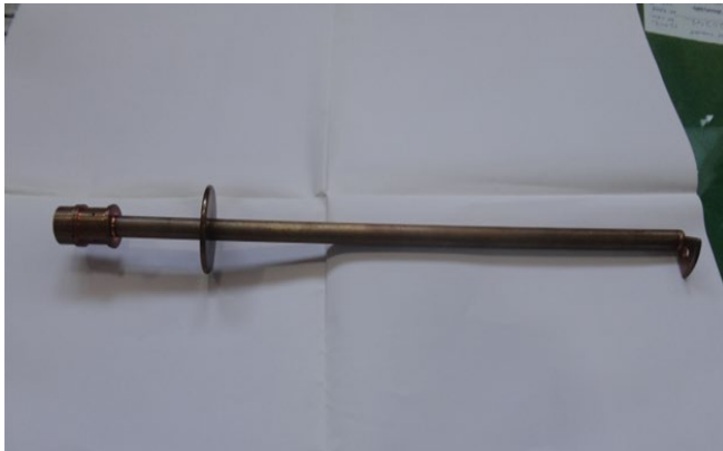
Inner conductor antenna
