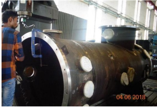
Machining of Vacuum Vessel Ports
