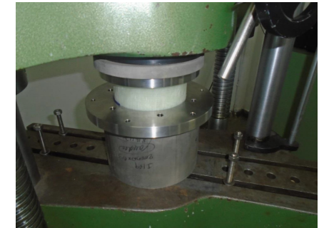
Testing of Support Port Assembly
