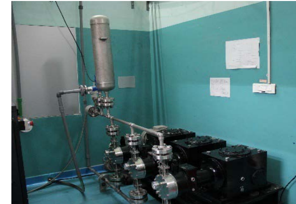
Hydraulically actuated diaphragm Pump
