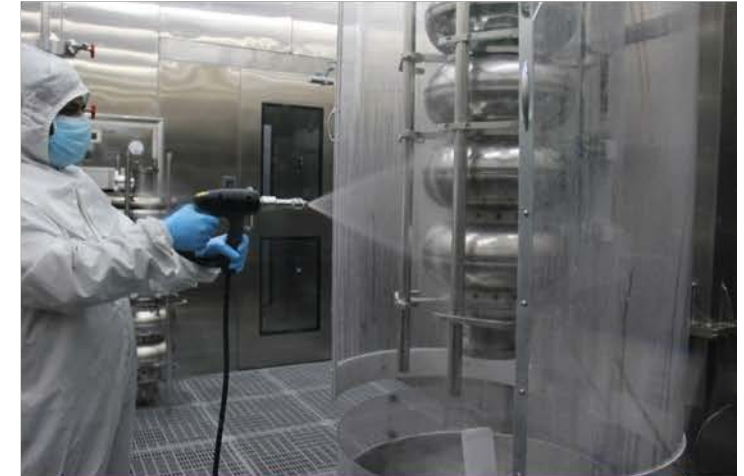
External rinsing of 5 cell 650 MHz cavity
