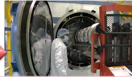
Degassing/ N-Doping @ 800° C – 3 hrs
