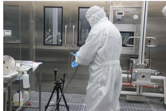
Hardware blow off using ionized nitrogen
