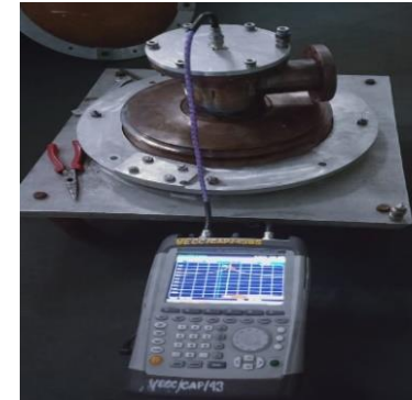
Frequency measurement of dumbbells, endgroups and dumbbell trimming
