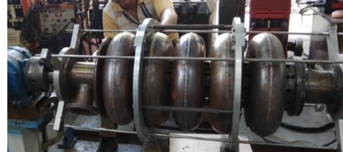
Copper prototype half-cells, sub-assemblies with welding fixture & welding of coupler port
