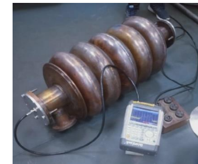
Frequency measurement of sub-assemblies and 5-cell LB650 copper prototype cavity
