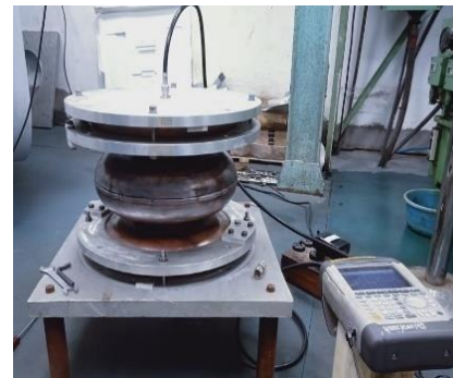
Frequency measurement of sub-assemblies and 5-cell LB650 copper prototype cavity
