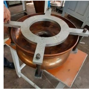
Copper prototype half-cells, sub-assemblies with welding fixture & welding of coupler port
