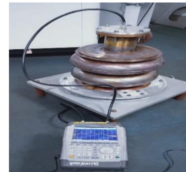
Frequency measurement of sub-assemblies and 5-cell LB650 copper prototype cavity
