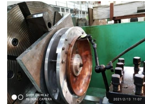
Frequency measurement of dumbbells, endgroups and dumbbell trimming
