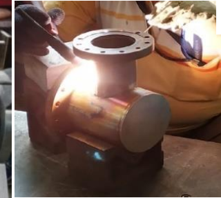
Copper prototype half-cells, sub-assemblies with welding fixture & welding of coupler port
