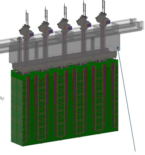
! Section of cryostat top lid with thermal insulation is not in the MS scope
