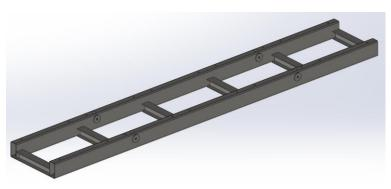
Welded frame made from rectangular stainless steel tubes, Ibeams and shaft hubs
