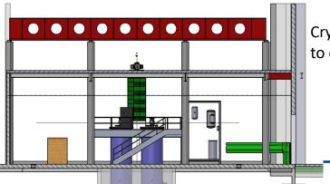
Cryostats located in pit to enable clearance
