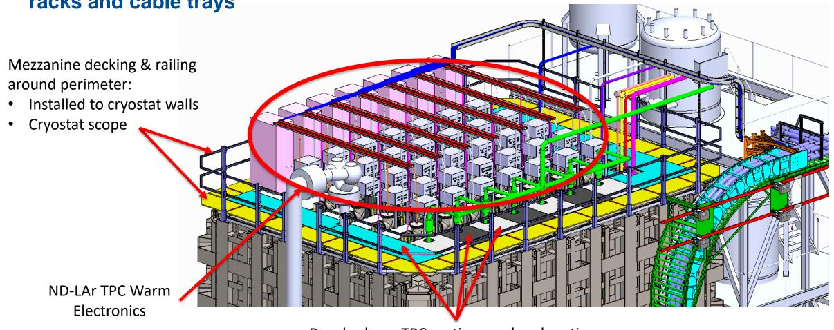
Panels above TPC sections and end sections are removable for access to feedthrough flanges or can be fully removed
