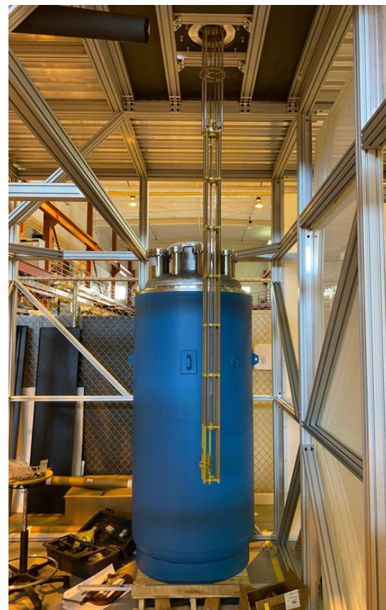
Periscope assembled in test stand
