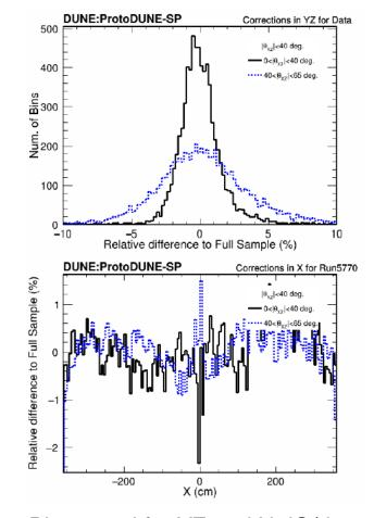
Plots used for YZ and X dQ/dx calibration to verify subsample deviations from the larger sample.
