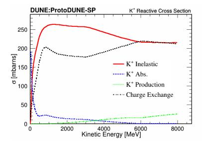
Total reactive cross section (left) and the exclusive cross sections (top) from <u>Geant4</u>. Plots produced using <u>Geant4RW</u>.
