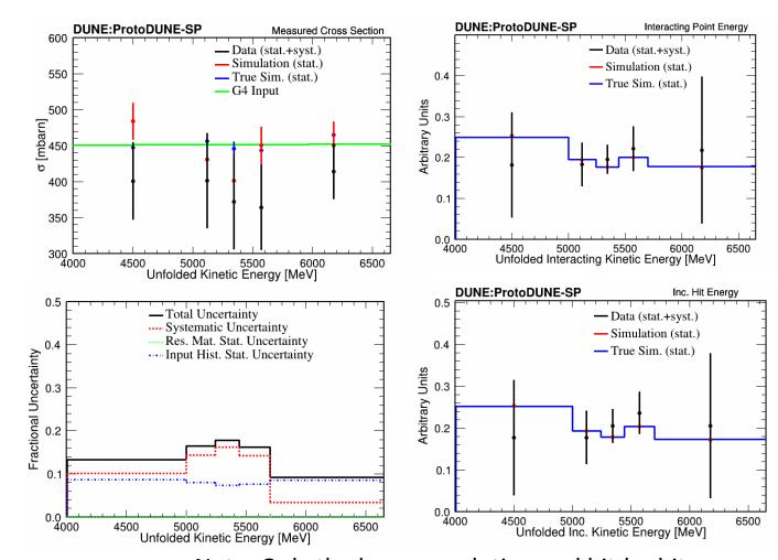
Note: Only the beam resolution and hit-by-hit calorimetry systematic uncertainties are used.
