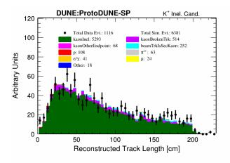
Reconstructed track length for Run 5770 and simulation of selected interacting events (same plot as the previous slide).
