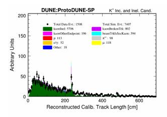
Reconstructed track length for Run 5770 and simulation of selected events.
