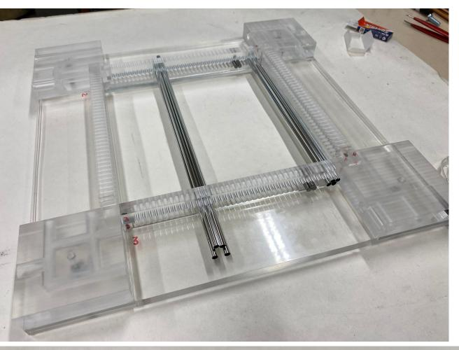
Residual tension on straw walls enough to support weight (validation of overpressure for assembly)
