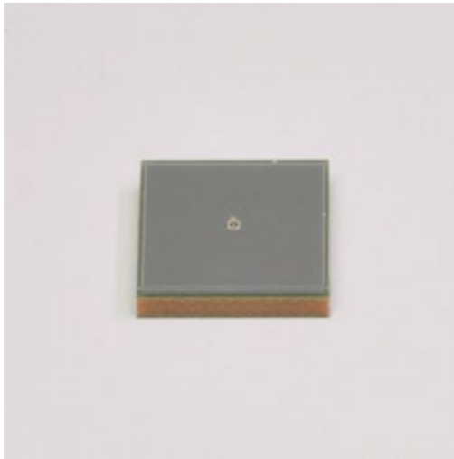
S14160-6050HS 6x6 mm 2 Pixel pitch: 50 μm
