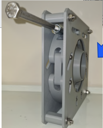
Remotely operable helium line connector Designed and prototyped by Year In Industry student
