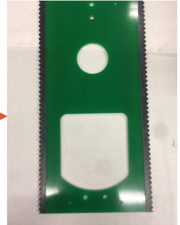
Wrap board after Tooth-Strip Assembly
