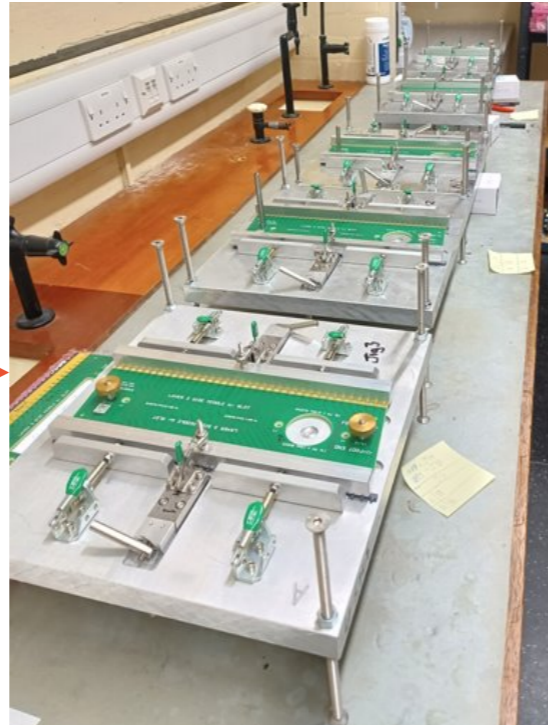
Tooth-Strip Assembly Jigs
