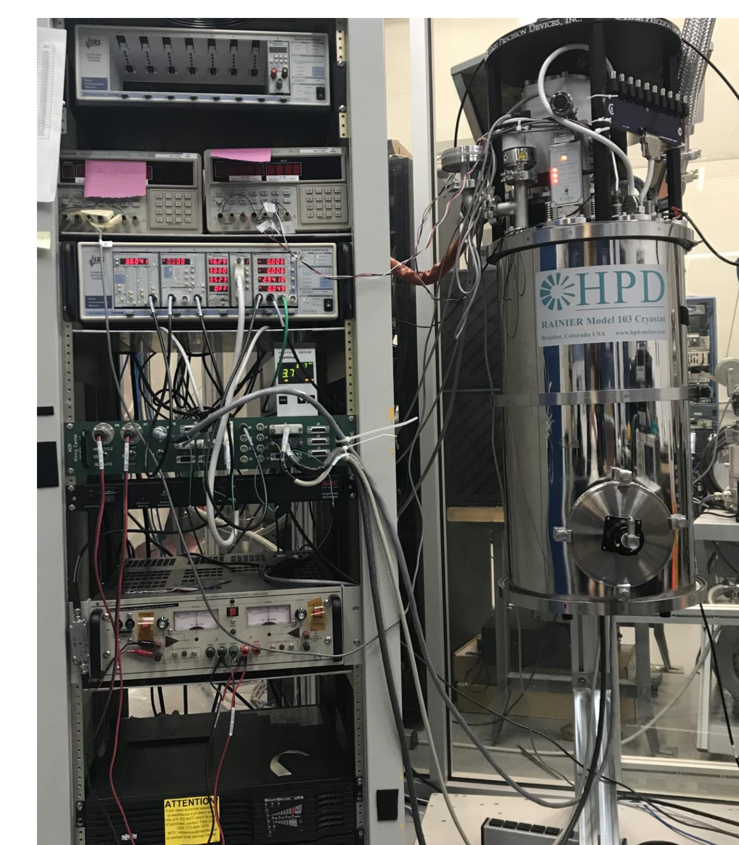
Fig 3. – On the right is the ADR with the SNSPD and amplifier board installed. On the left is a rack containing temperature, pressure, current, and voltage measurement devices as well as a power supply for the ADR magnet and an uninterruptible power supply and battery pack that aid in preventing the magnet from quenching.
