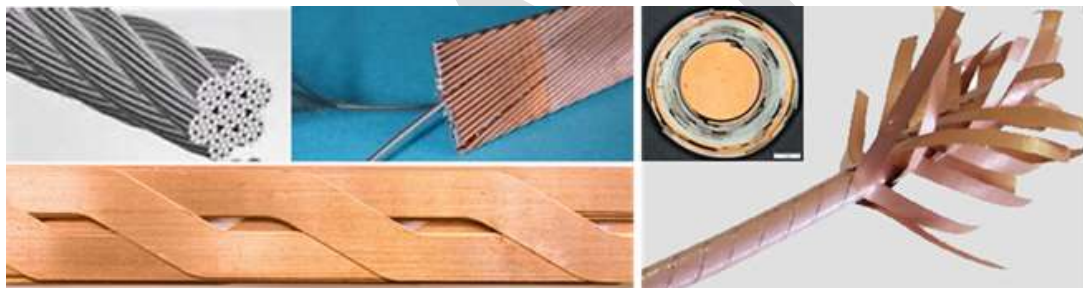
Figure 5.2 . Rope-type (top left), Rutherford-type (top right) and Roebel-type (bottom) multistrand superconducting cables. Add CORC, etc.
