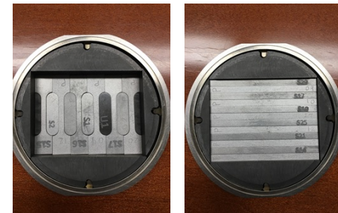
Be specimens assembled in BLIP capsule
