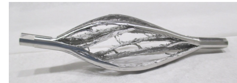
Iridium target tested at CERN's HiRadMat facility
