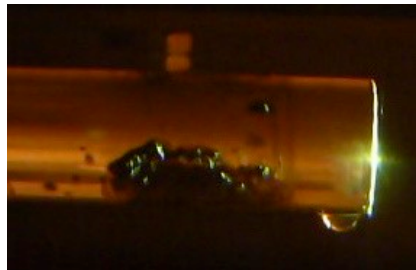
MINOS NT-01 target containment water leak (FNAL)
