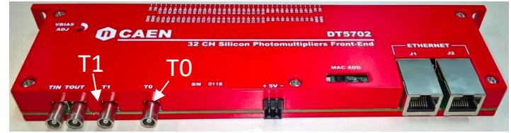
Picture of one of the FEBs used for the CRT system
