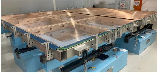
Wire Plane 3 readout wire planes ~11000 wires
