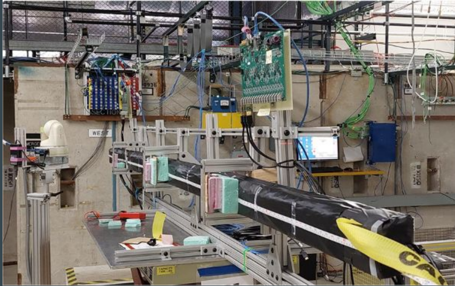
Fermilab test beam (left) and quad-counter configuration (right) with proton beam going from left to right. Wire chambers are located to the left (Station 1 & Station 2) of pictured quad-counters.
