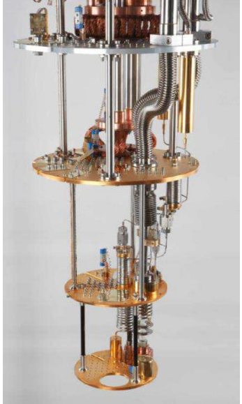
Small fridges Mixing chamber diameter ~150mm Minimum temperature ~25 mK
