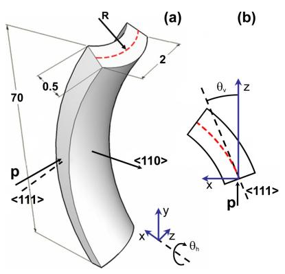
Crystal bending is accomplished through anticlastic deformation
