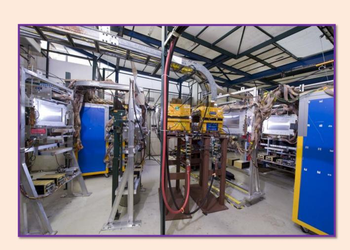
At the Fermilab Test Beam Facility: 16 GeV incident  $\pi$  beam on Cu followed by collimator, spectrometer, and time of flight system
