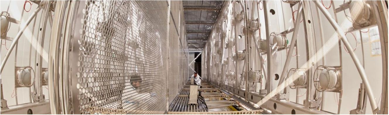
**Figure 5.** Picture of a ICARUS T300 module during the overhaul period at CERN. The module is composed of two TPCs, divided by the common central cathode. The PMT systems of the two TPCs are visible at the sides, where the anode plane is located aswell. Field cages, located at the top and bottom of the TPCs, can be seen.
