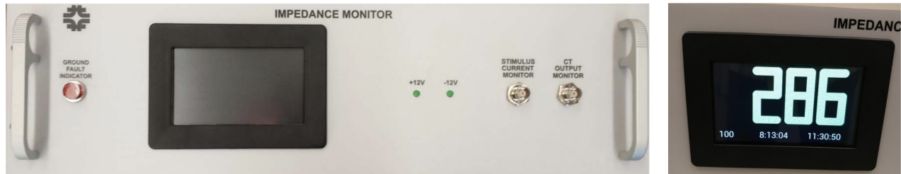
Figure 6. GIZMo front panel. The resistance numerical value is shown on the right-hand-side.
