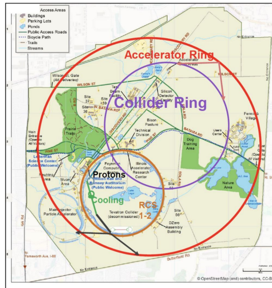
Figure 2: A schematic view of the Fermilab site and the layout of a possible complex for the Muon Collider site-filler.
