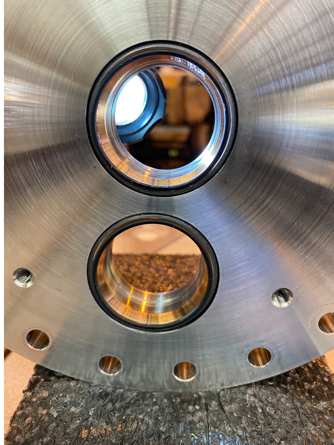
After cleaning w/ waterspot treatment on all quartz windows (inner and outer surfaces)
