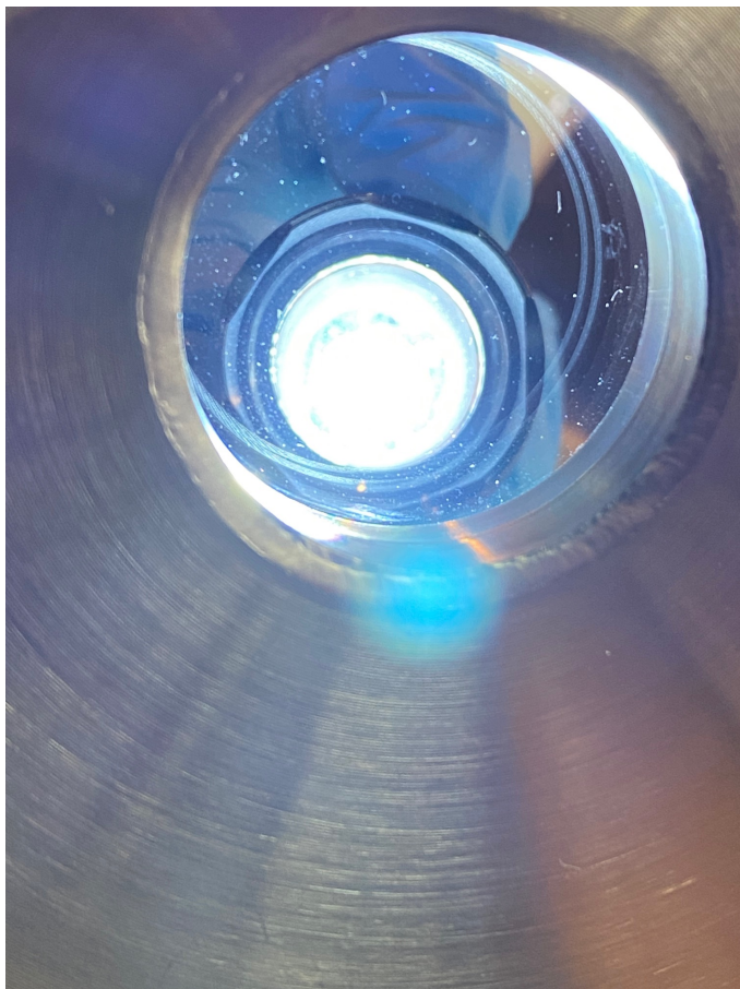
Significant dust and a spot on outer edge of beam window. Camera viewport also looked dusty.
