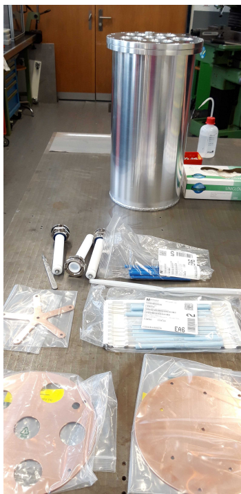
Assembly stages of the HV filter PFD-5
