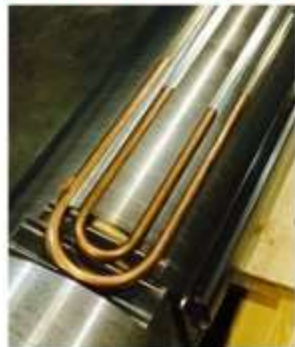
Water line channels machined
