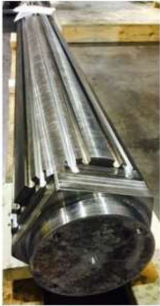
Water line channels machined
