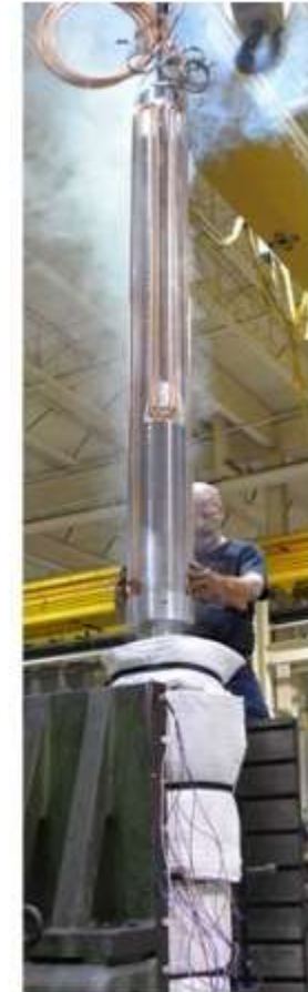
Core shrink-fit into aluminum sleeve
