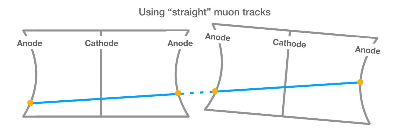
Correct modules to a common reference frame
