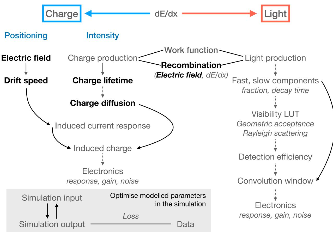
Simultaneously fit multiple parameters of the bulk LAr detector in the simulation from a noiseless closure test
